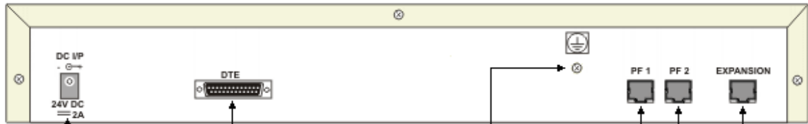
DC Power Input Socket To external power supply unit.
